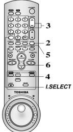
To record from other connected equipment In step 3, press *I.SELECT* to switch the display as follows: L1: To record via the LINE IN 1 jacks on the rear panel. L2: To record via the LINE IN 2 jacks on the front panel.
